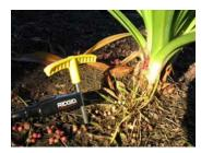
Dry sandy soil provides more of a challenge. In dry, sandy soil the resistance to current flow causes a lower locatable signal. Water can be added to very dry soil to improve the grounding and lower resistance. Keep a mixture of Gatorade and Water in your vehicle for this purpose.
