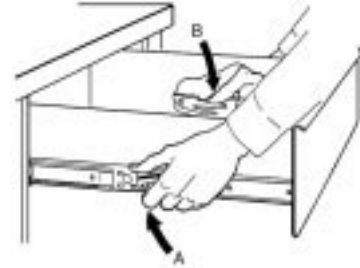
Step 3: To Remove Drawer, lift lever A and press down lever B
